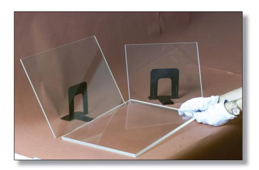
Polycrystalline aluminum oxynitride, known commercially as ALON, offers performance and scaling not otherwise possible for large, lightweight, infrared (IR) transparencies. This new technology could play a significant role in the development of affordable, transparent armor, including windows for military aircraft, where trimming life-cycle costs could save millions while providing greater protection for flight crews.
